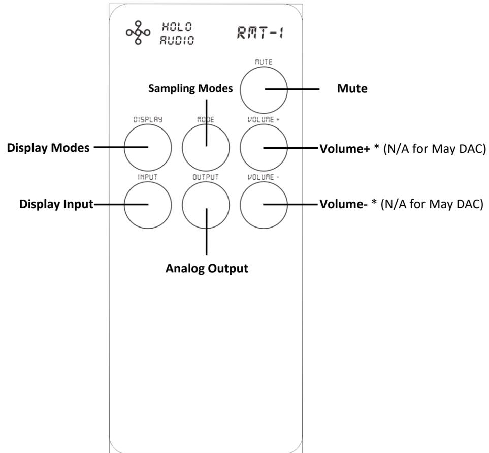
\*This is a universal HOLO AUDIO remote. Volume (+/-) is not applicable to the “梅” May DAC as there is no pre-amp built in, will work simultaneously with other HOLO Audio branded products i.e. pre-amps and head-amps.
