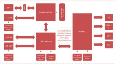
When the USB-IN is effectively connected, the USB DDC will be connected to the USB-IN and disconnected from the USB processor; I<sup>2</sup>S, COAX-1, COAX-2, OPT, AES will simultaneously output the audio signal from the USB-IN.
