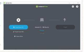
Select the desired system image (.img file) in the BalenaEtcher-Portable software under "Flash from file", select the corresponding TF drive letter under "Select target", and then select "Flash!" to start writing to the system. A dialog box will appear asking if you are sure, select "Yes".
